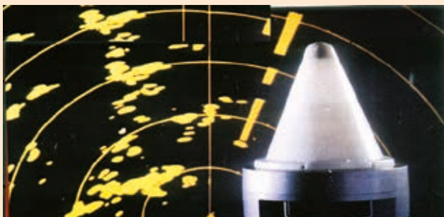
Racon along with display of its Character on a Radar screen
