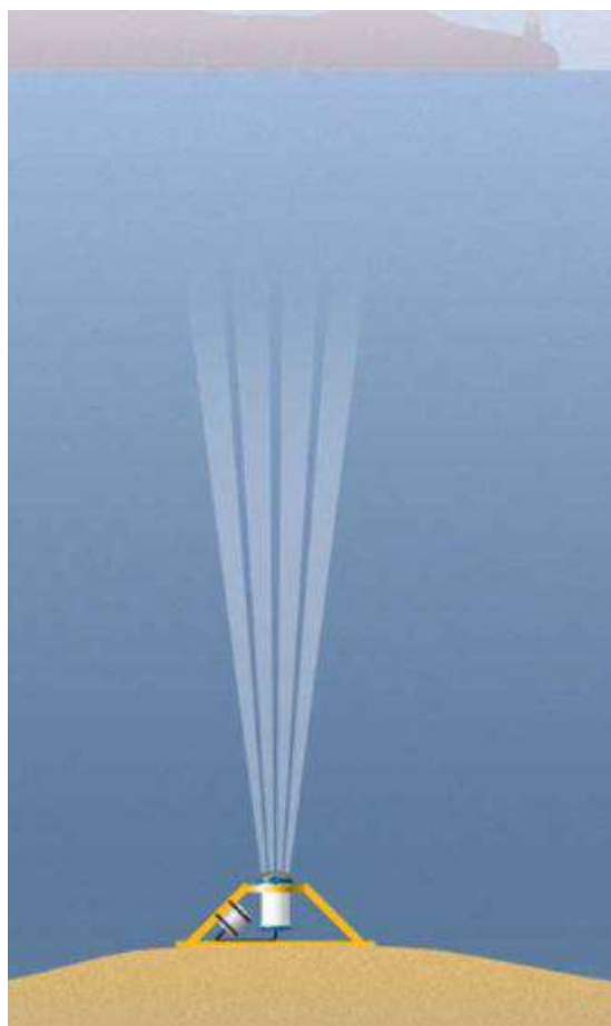
Fig. 4.7 Typical graphical picture showing ADCP bottom mounting arrangement
