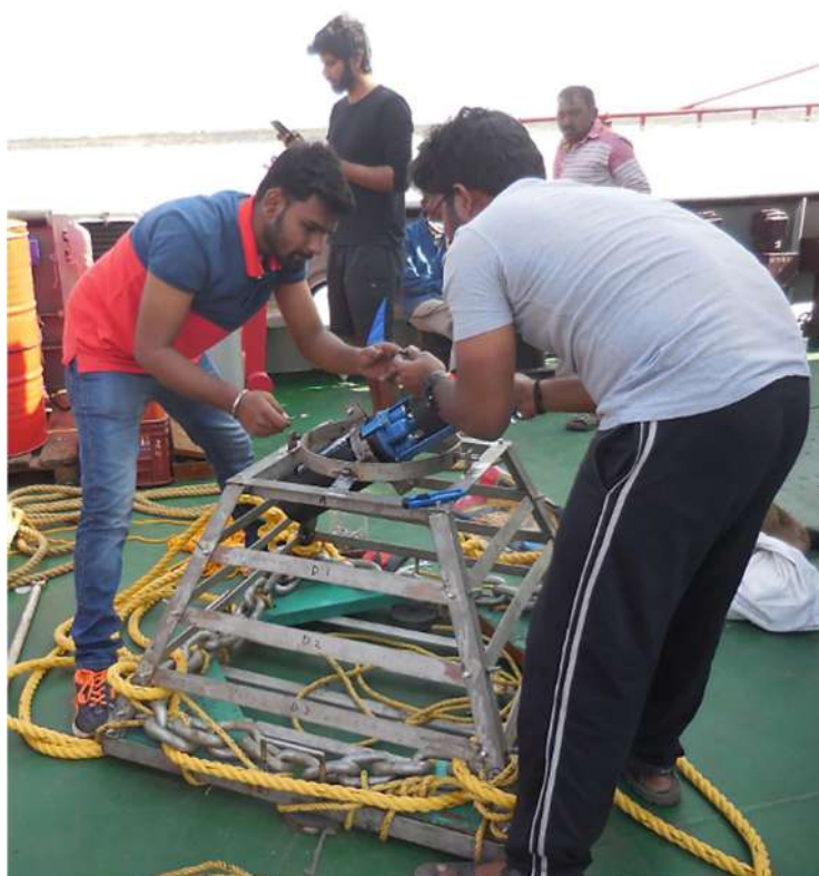
Fig. 4.42 RCM fitted to frame (with dead-weights)
