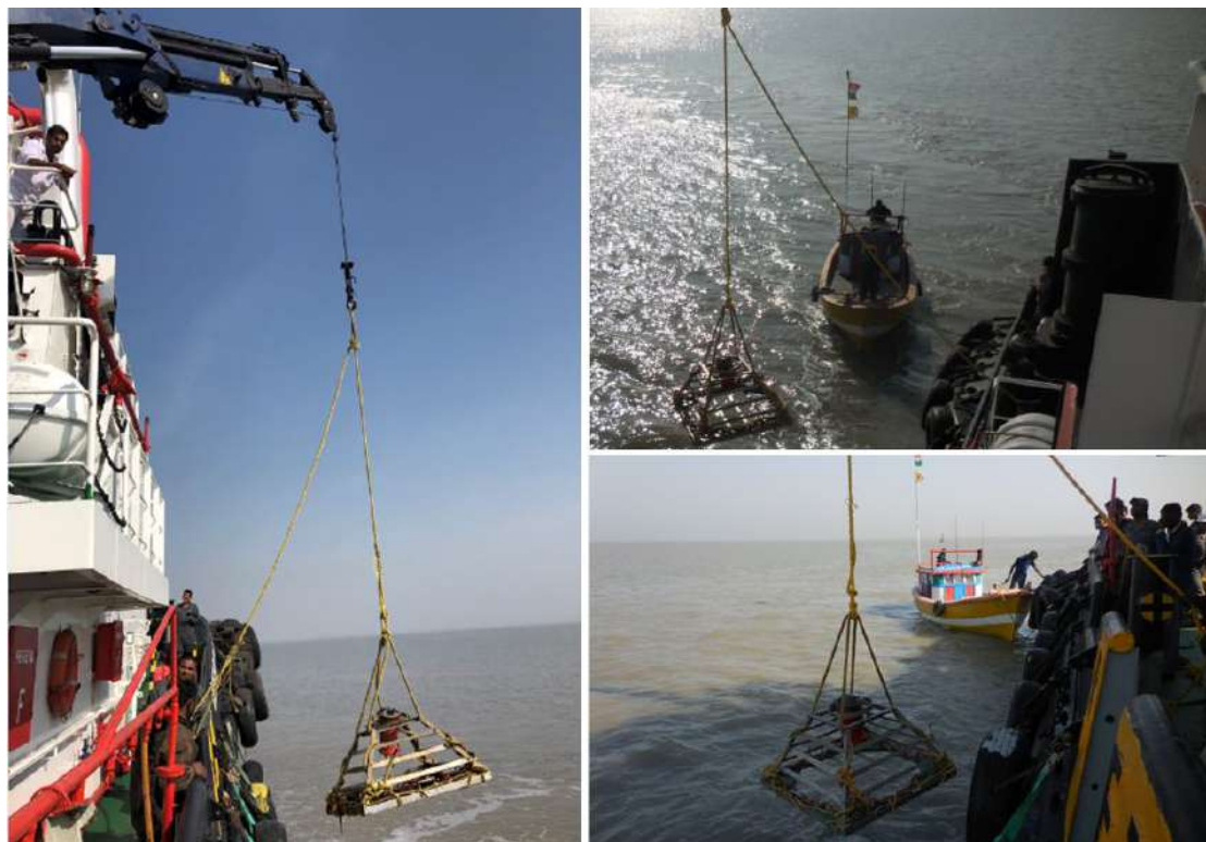
Fig. 4.30 Deployment of ADCP with the help of hydraulic crane installed in tugboat
