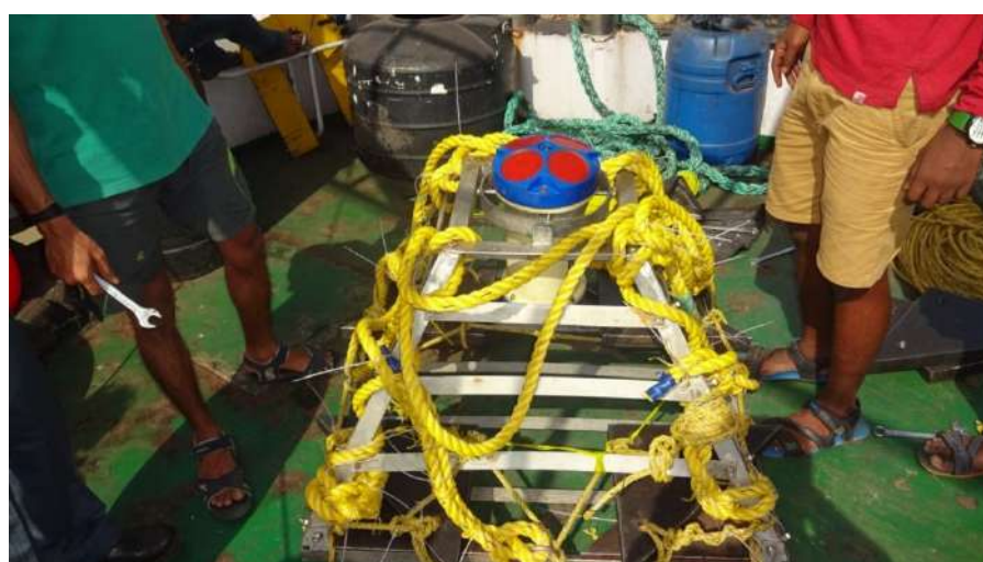
Fig. 4.6 ADCP set for deployment with all the arrangements
