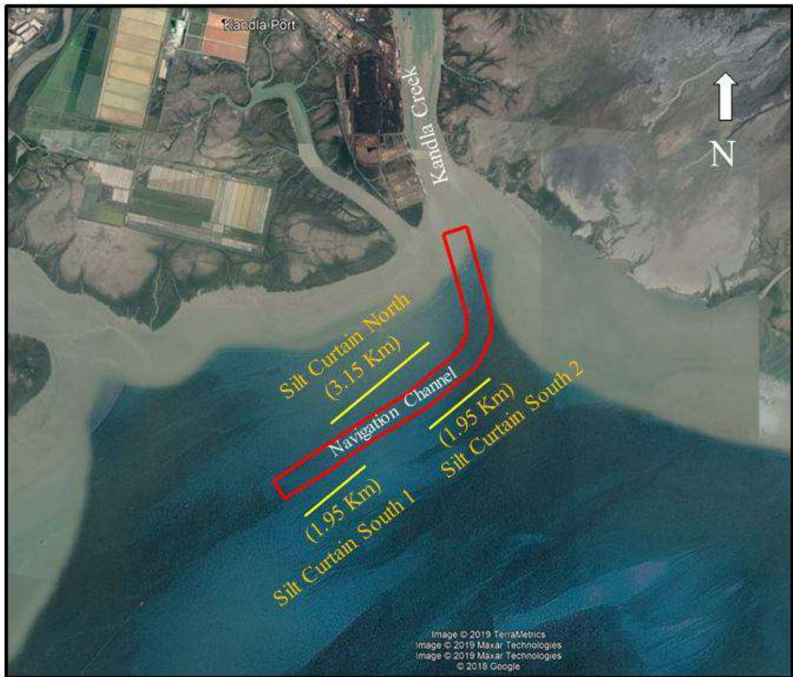
Fig. ES2 Suggested silt-curtain option for reducing siltation in navigational channel
