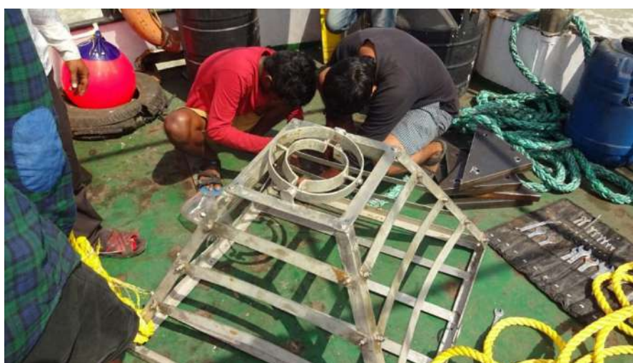
Fig. 4.5 Assembled frame with gimbal on the top
