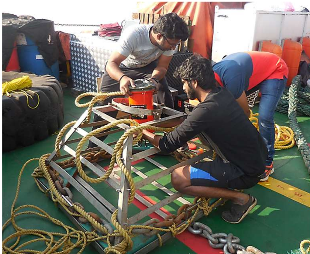
Fig. 4.29 Clamping of ADCP in detachable frame (with dead weights)
