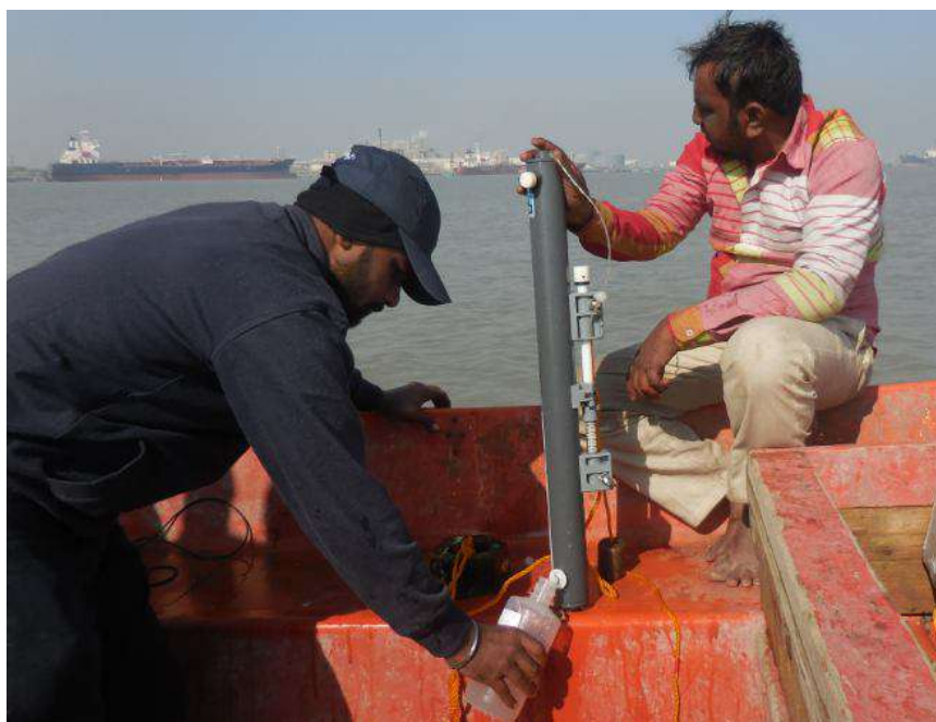
Fig. 4.52 Collected water sample transferred to collection bottle
