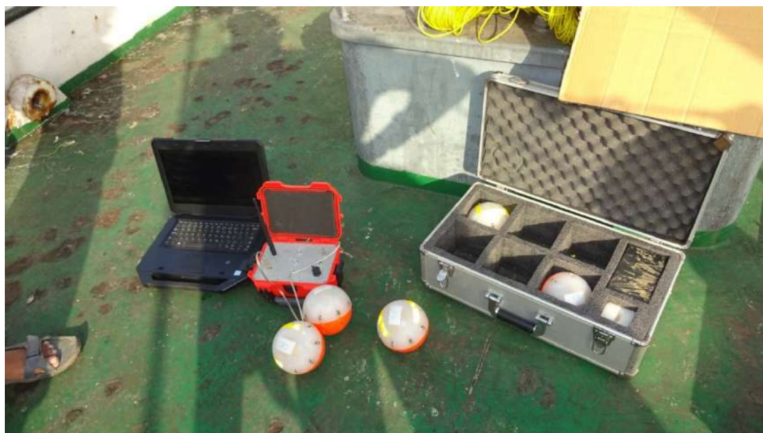
Fig. 4.24 Typical floating drifters with the base station kit
