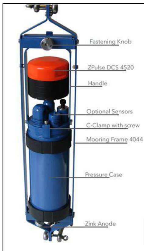
Fig. 4.11 Typical view of RCM with all sensors
