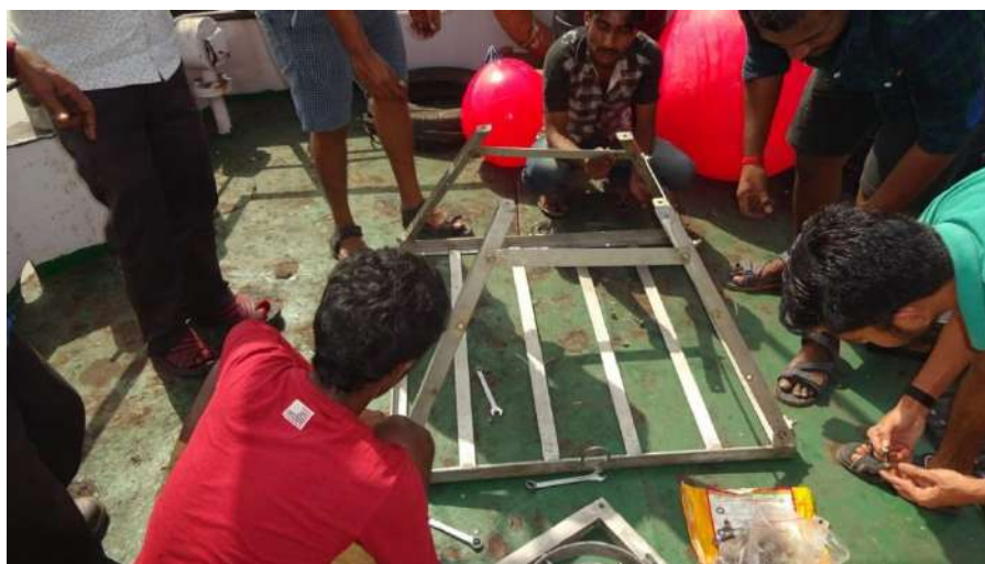
Fig. 4.4 Assembling the frame for ADCP deployment
