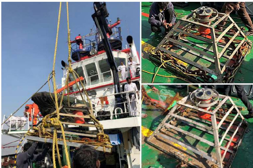
Fig. 4.32 Retrieval of the instrument with the help of crane from tugboat
