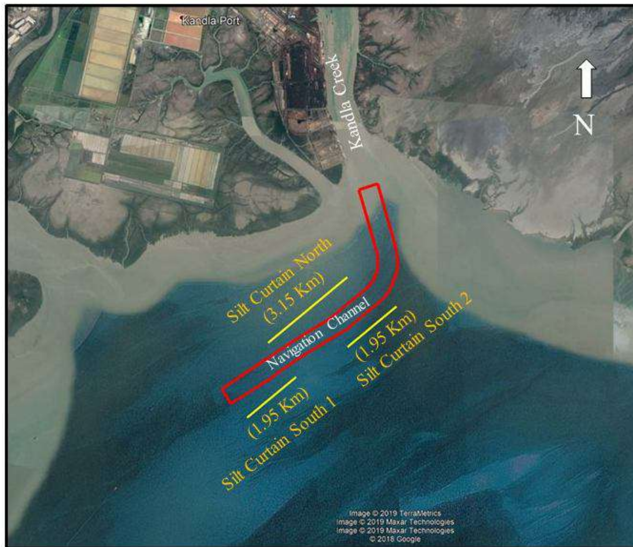
Fig. 3 Suggested silt-curtain option for reducing siltation in navigational channel
