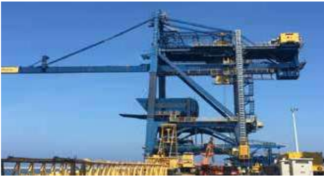
Ship Un-loader at Modified Iron Ore Terminal to also handle Coal
