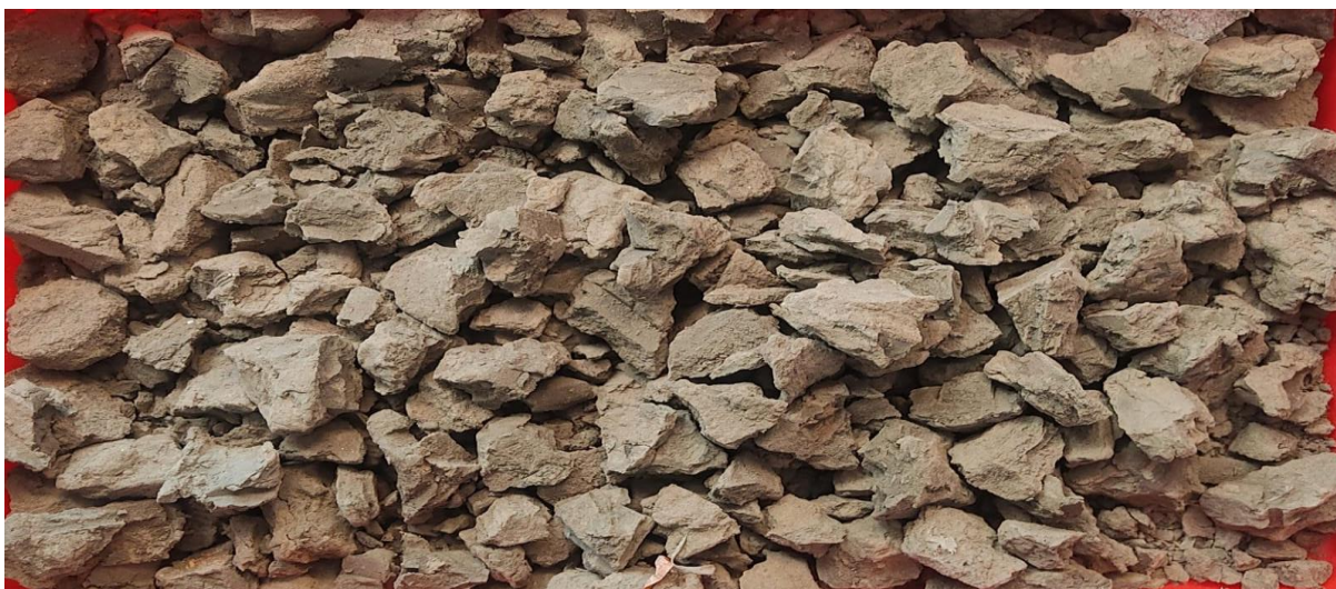
Figure 12. Aggregates from the desiccated MDS in the Confined Disposal Facility
