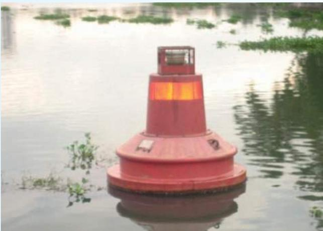
Solar Powered FRP Buoy installed in NW-3
