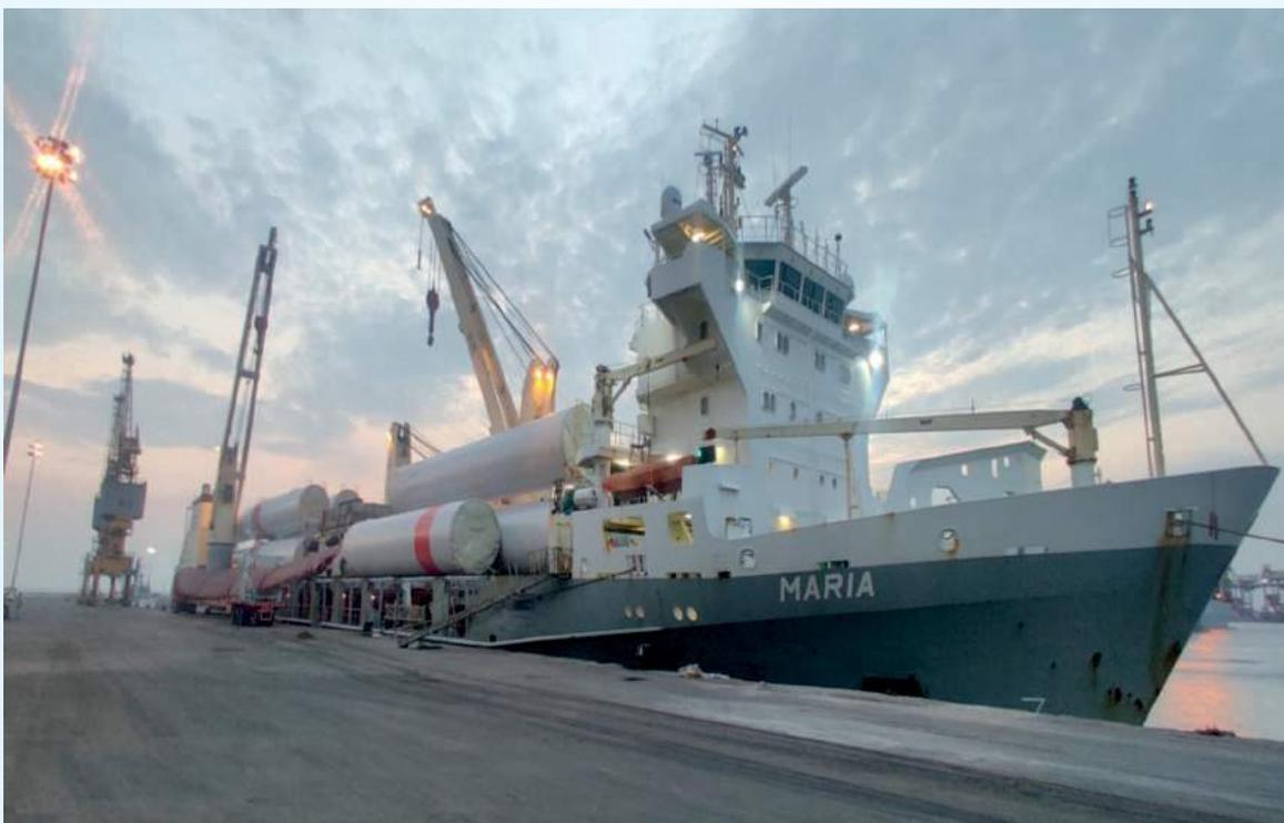
Windblade being loaded into the Ship 'M.V Maria' using Ship's hydraulic
