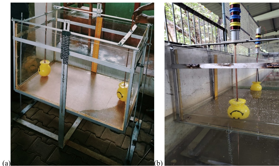
Fig 7: (a) Floating breakwater with built-in buoys (b) Floating breakwater with built-in buoys connected to linear inductance generator.
