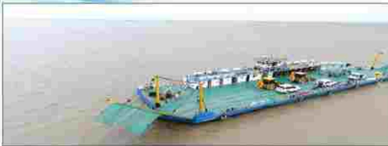
Figure 14: NW-1 Ro-Ro cargo handling operation
