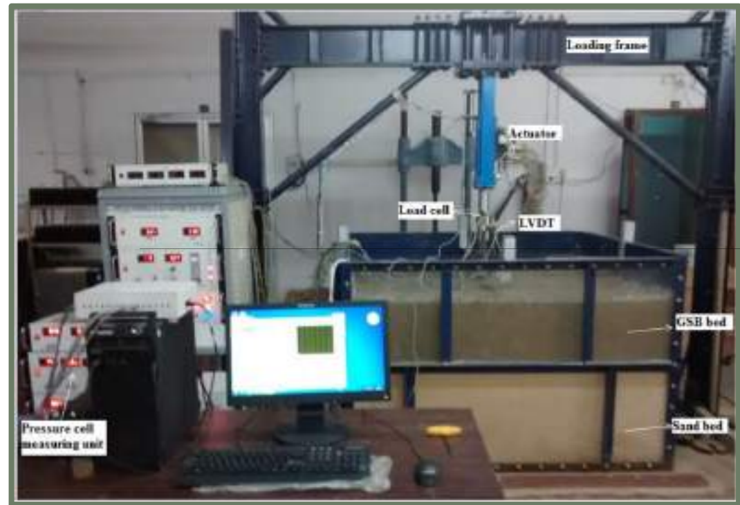
Plate load test setup with data acquisition system
