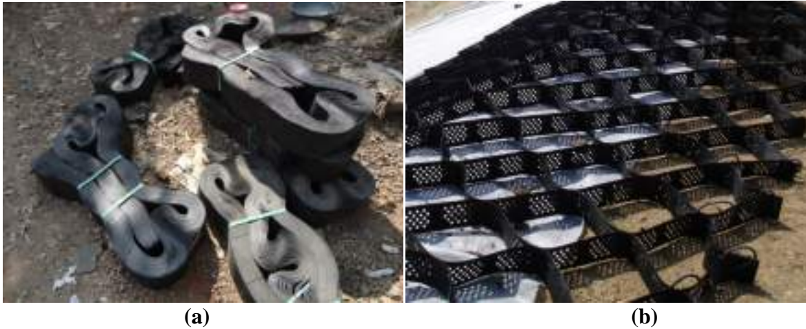
Figure 3.5 Geocell (a) closed form as supplied from factory, (b) open form ready for infilling
