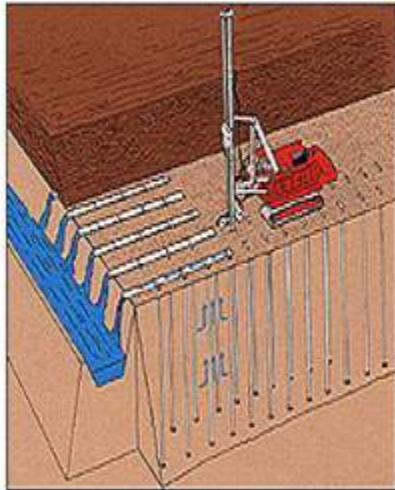
3D View of Band Drain Stabilised Bed
