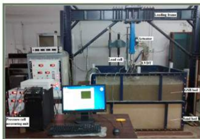
Plate load test setup with data acquisition system
