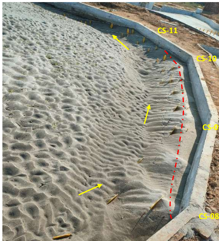
Fig. 7.16(b) Residual bed after running the model at 105600 m 3 /s discharge with vane
