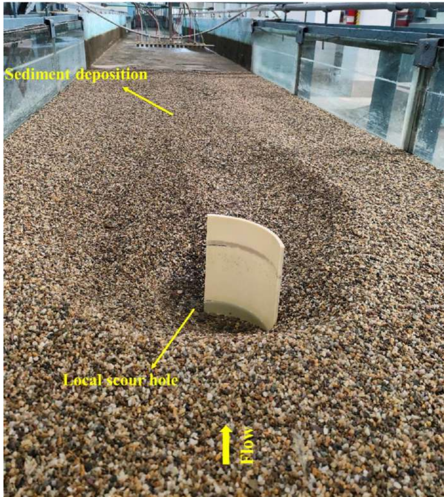
Fig. 3.13b Photographic image of equilibrium scour bed condition after the experimental run for Q = 0.082 \text{ m}^3/\text{s} , H = 0.045 \text{ m} , \alpha = 0^\circ
