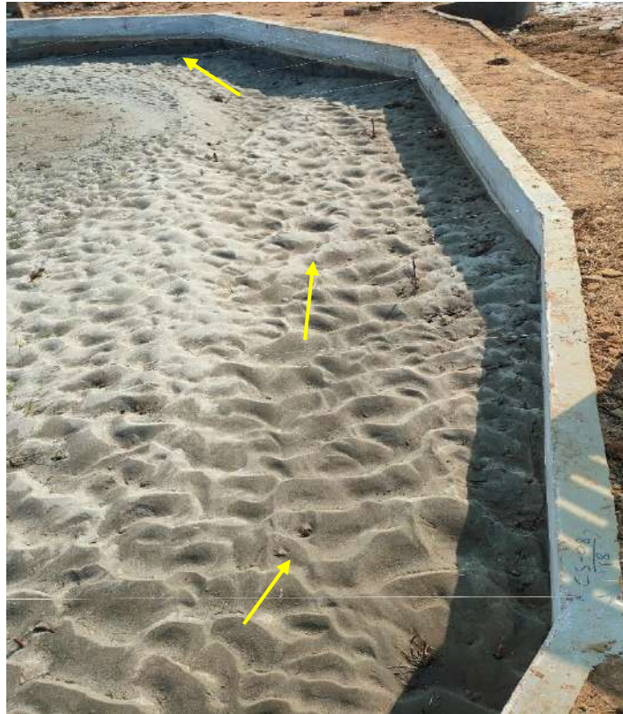
Fig. 7.14(a) Residual bed after running the model at 52800 m 3 /s discharge w/o vane
