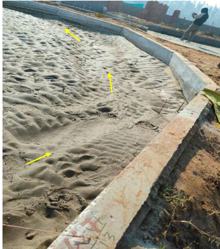
Fig. 7.16(a) Residual bed after running model at 105600 m 3 /s discharge w/o vane
