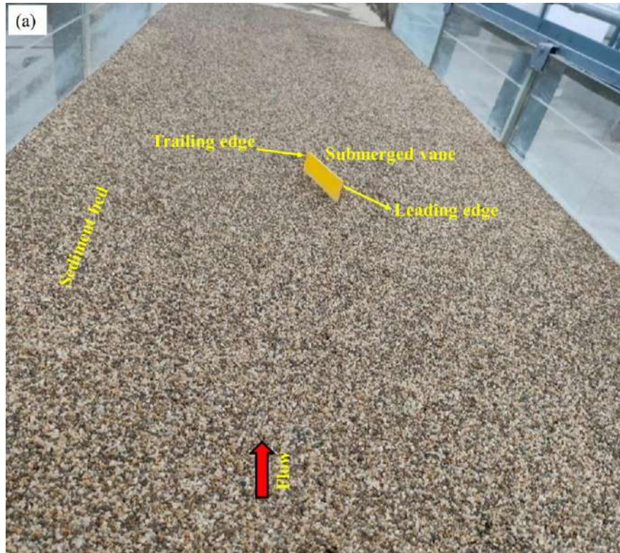
Fig. 3.11a Photographic image of the rectangular vane before experiment run
