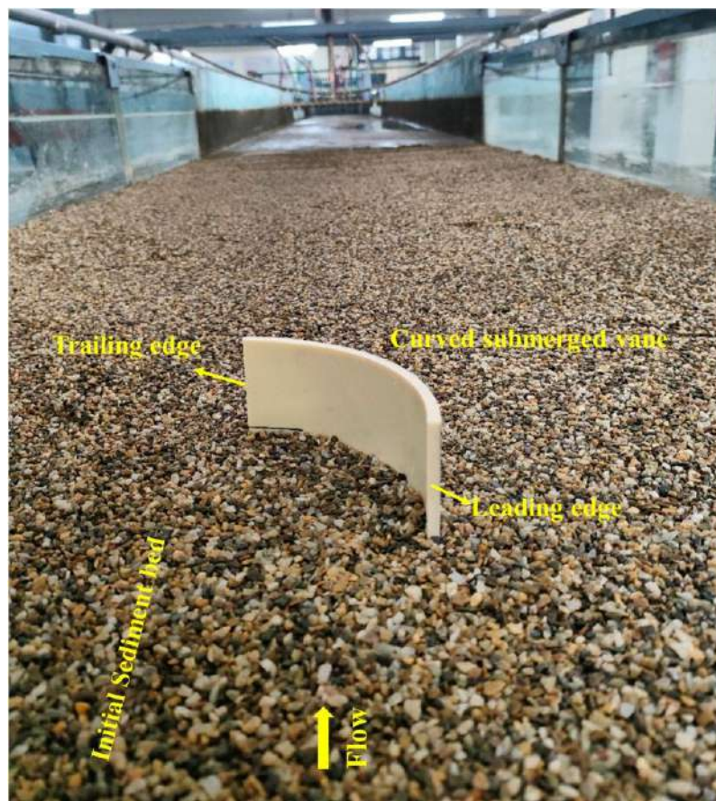
Fig. 3.13a Photographic image of the curved vane before experiment run
