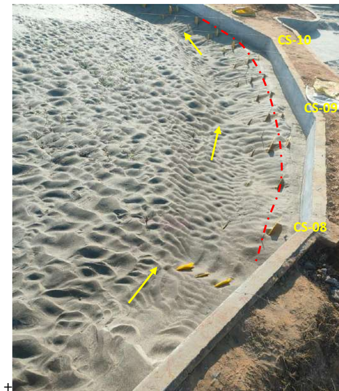
Fig. 7.15(a) Residual bed after running the model at 79200 m 3 /s discharge w/o vane
