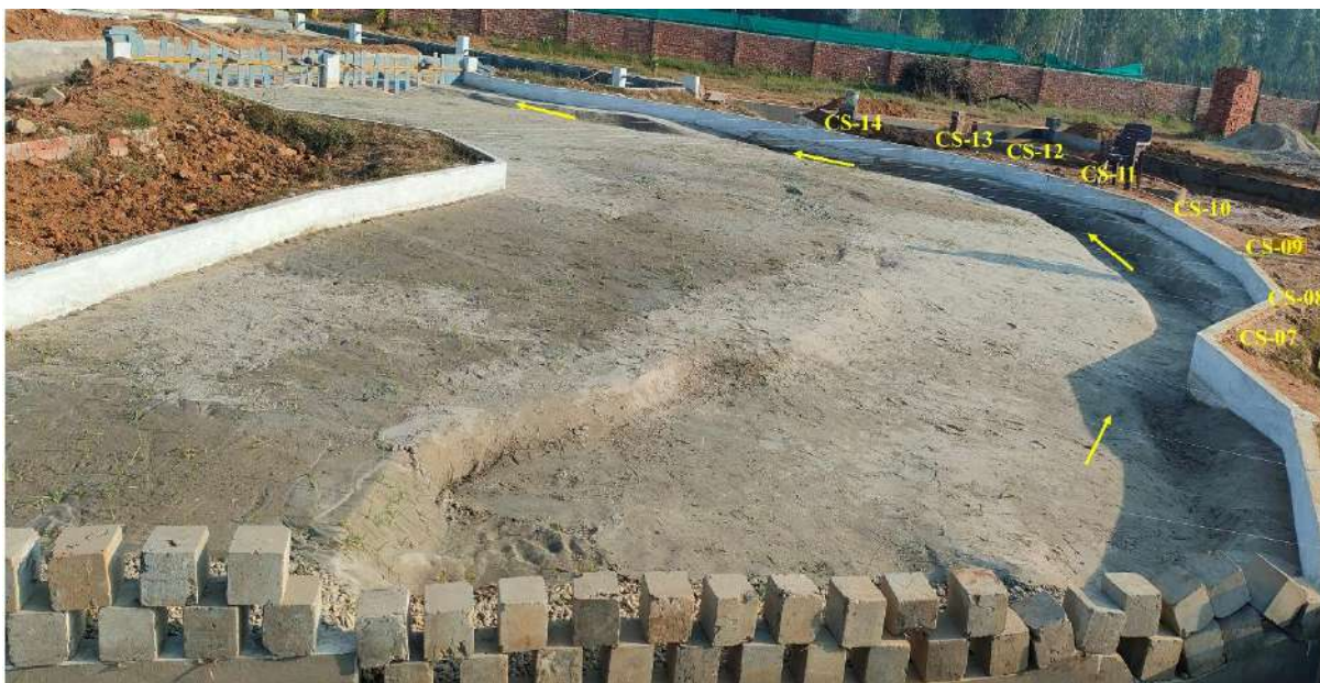
Fig. 7.5(a) Physical model of Ganga river at Bhagalpur without vane
