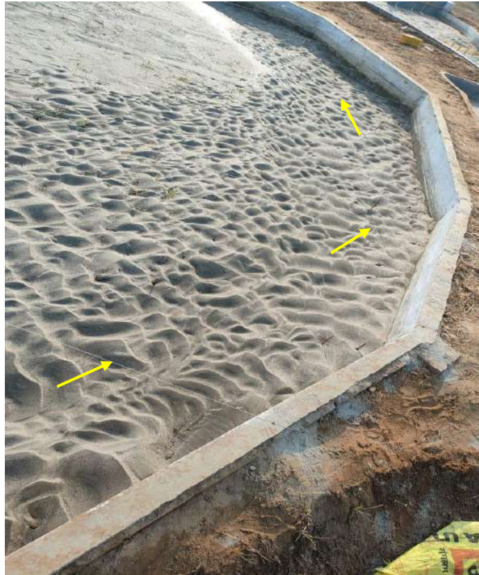
Fig. 7.13(a) Residual bed after running the model at 26400 m 3 /s discharge w/o vane
