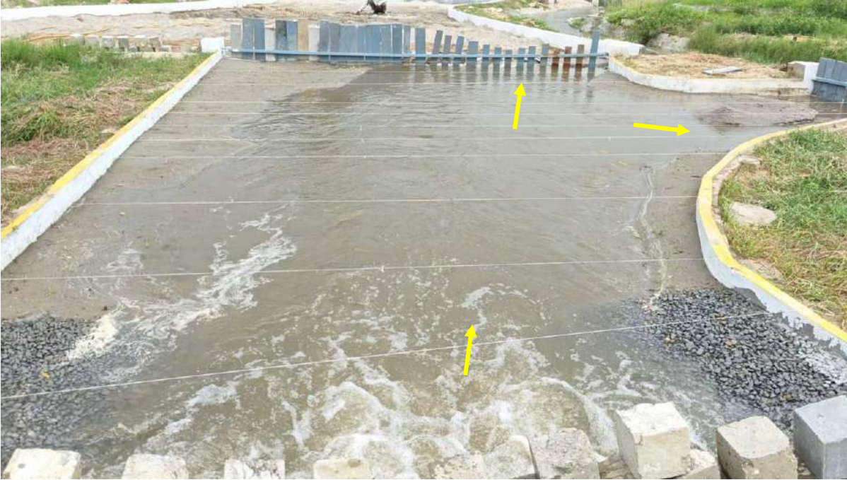
Fig. 8.10g Flow pattern for 41500 m 3 /s discharge with submerged vanes
