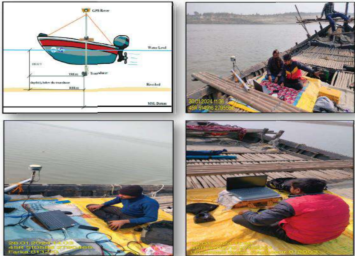
Fig. 7.4(c) Showing the Hydrographical survey through Echo-Sounder, Photographs
