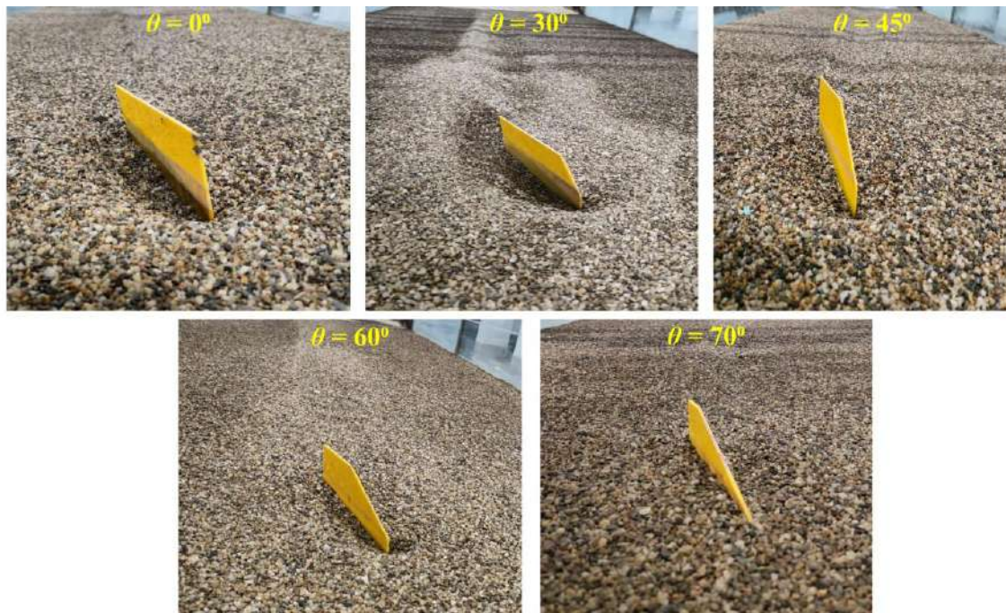
Fig. 3.12 Scour hole geometry as observed during experimentation for various shape of bevel submerged vane under Q = 0.082 \text{ m}^3/\text{s} , H = 0.045 \text{ m} , \alpha = 20^\circ
