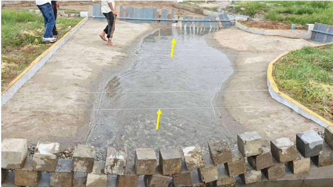
Fig. 8.7a Flow pattern for 8839 m 3 /s discharge under existing condition
