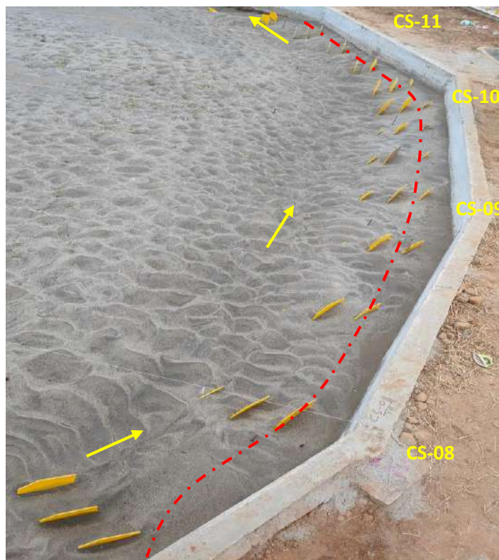
Fig. 7.14(b) Residual bed after running the model at 52800 m 3 /s discharge with vane
