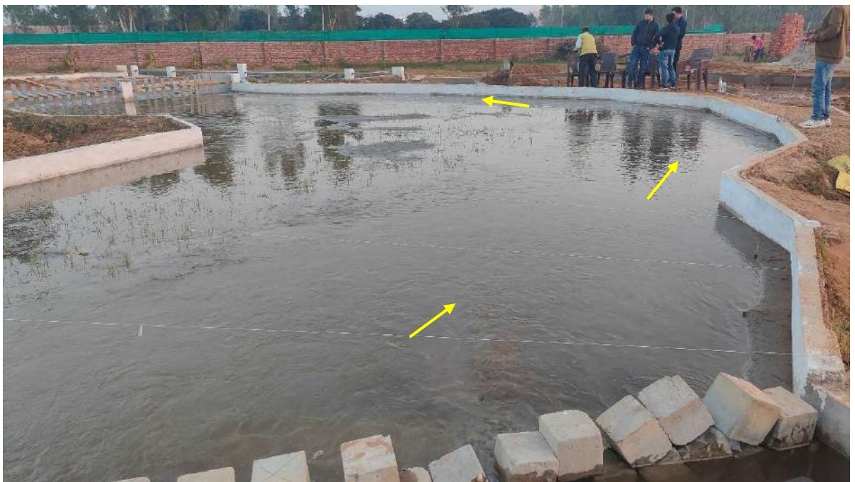
Fig. 7.8 (b) Flow conditions for 52800 m 3 /s discharge
