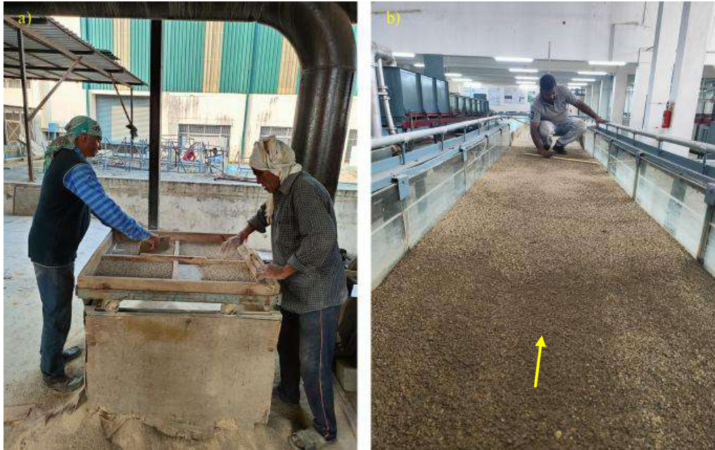
Fig. 3.3 Photography shows a) sediment sieve and b) sediment bed preparation
