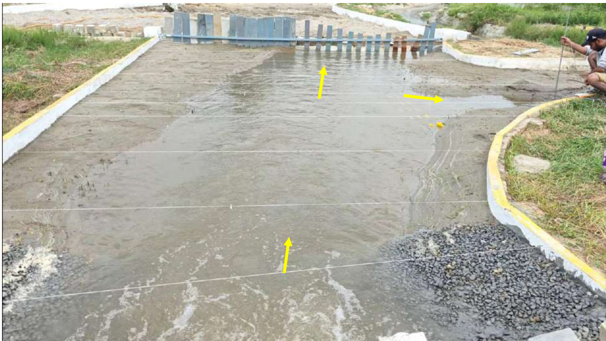
Fig. 8.10d Flow pattern for 24218 m 3 /s discharge with submerged vanes
