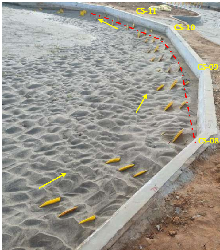
Fig. 7.13(a) Residual bed after running the model at 26400 m 3 /s discharge w/o vane
