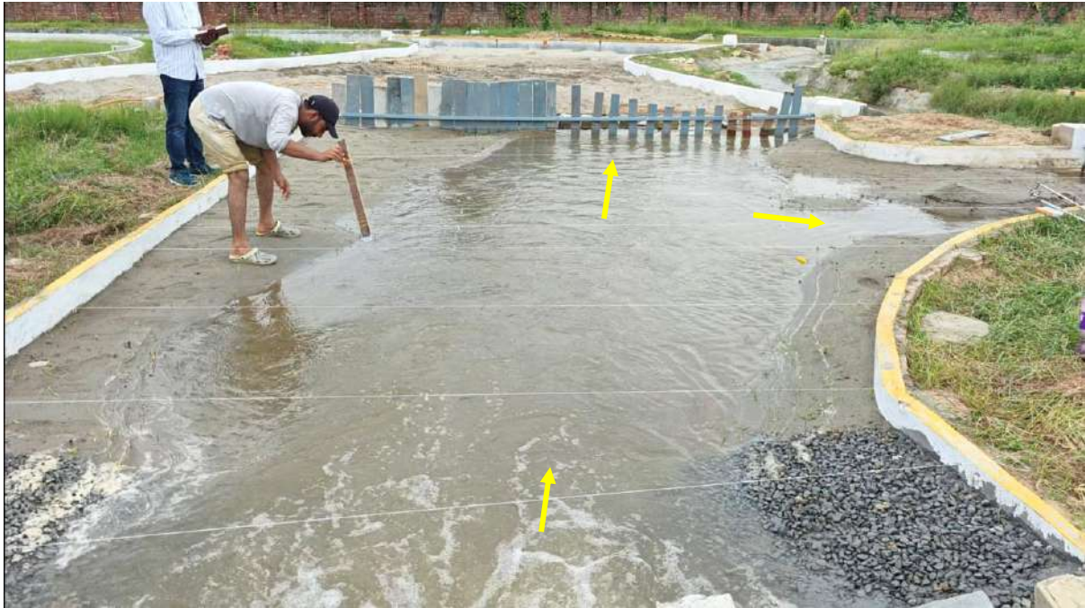
Fig. 8.10e Flow pattern for 30,052 m 3 /s discharge with submerged vanes
