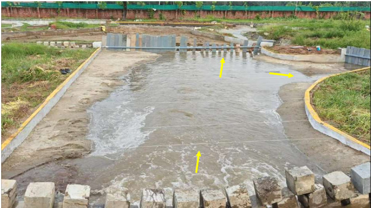
Fig. 8.7f Flow pattern for 35355 m 3 /s discharge under existing condition
