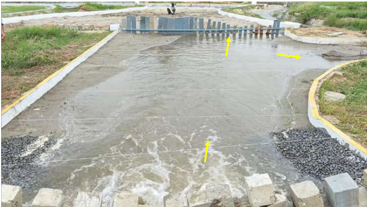
Fig. 8.10f Flow pattern for 35,355 m 3 /s discharge with submerged vanes
