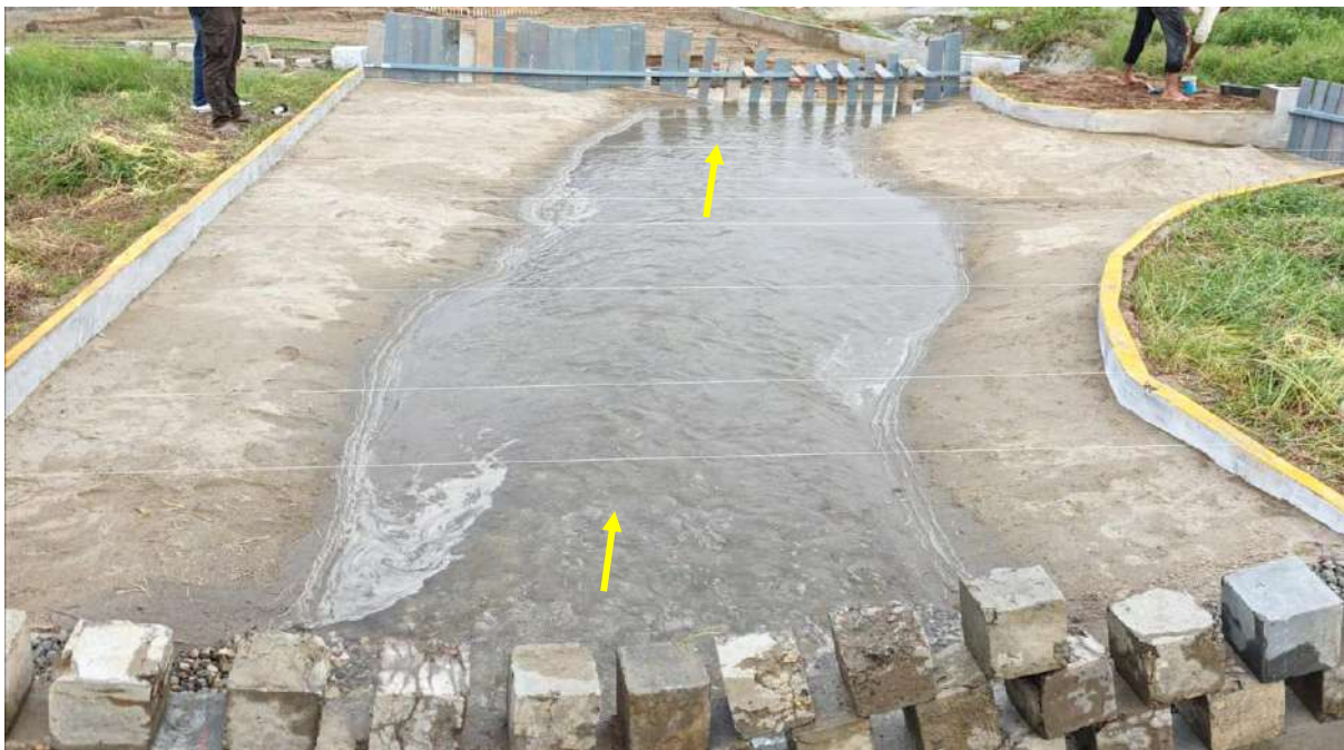
Fig. 8.7b Flow pattern for 14142 m 3 /s discharge under existing condition
