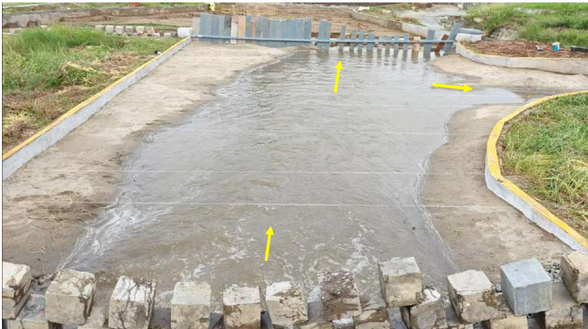
Fig. 8.7d Flow pattern for 24218 m 3 /s discharge under existing condition
