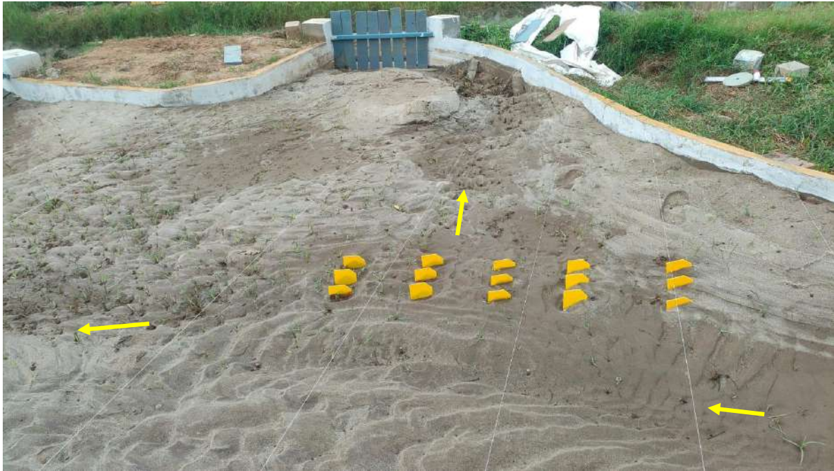
Fig. 8.13b Residual bed after running the model under submerged vane condition
