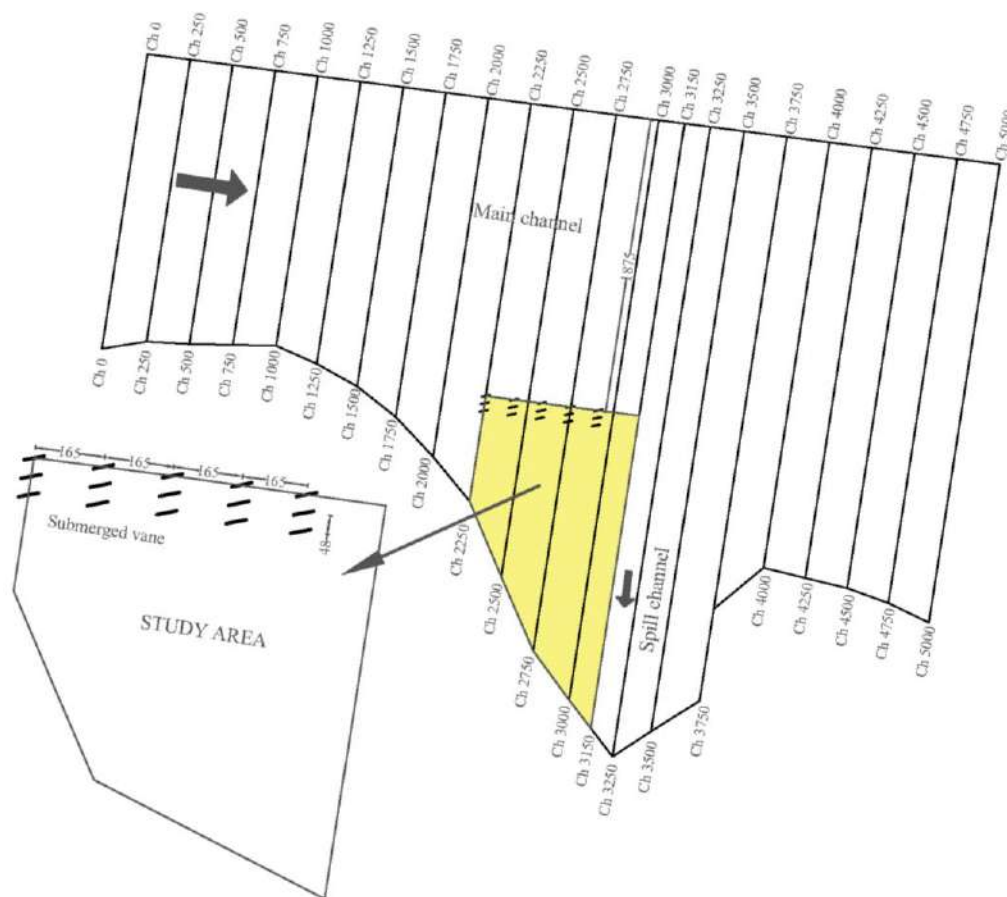
Fig. 8.6 Position of the installed submerged vanes in the model. The yellow-shaded area represents the region where bed elevation measurements were taken.
