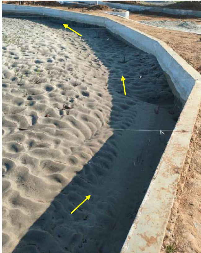
Fig. 7.15(a) Residual bed after running the model at 79200 m 3 /s discharge w/o vane
