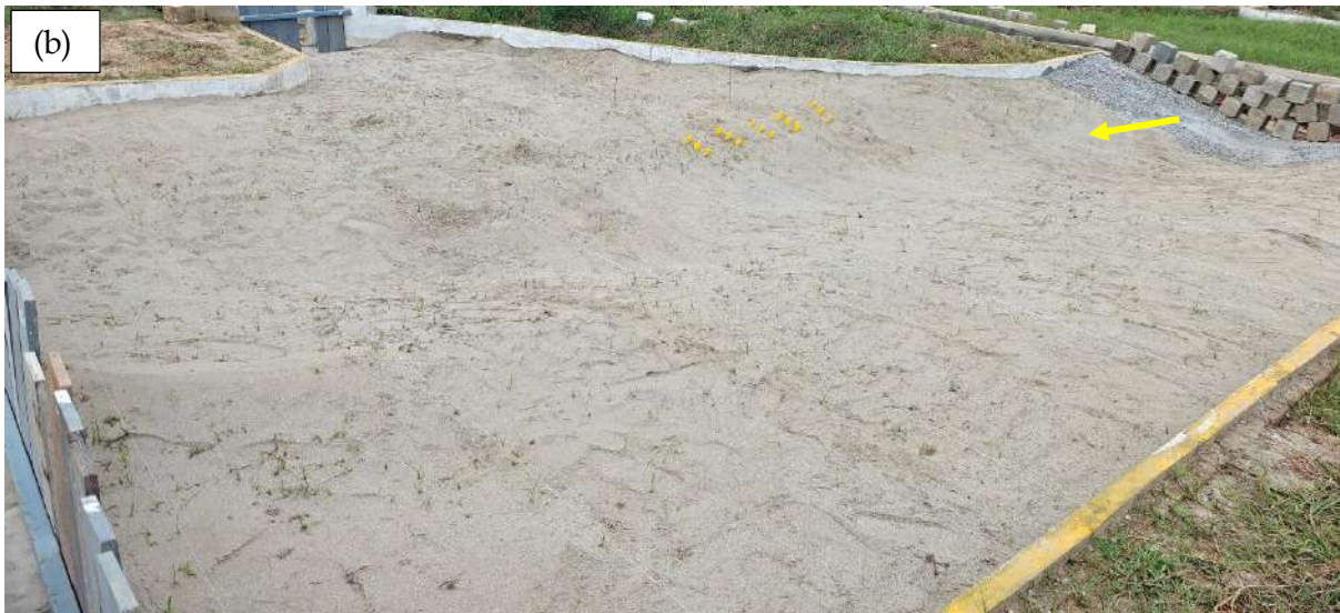
Figs. 8.9a-b View of the model under dry conditions with submerged vanes
