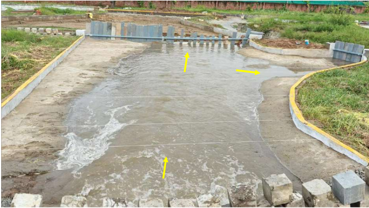
Fig. 8.7e Flow pattern for 30,052 m 3 /s discharge under existing condition
