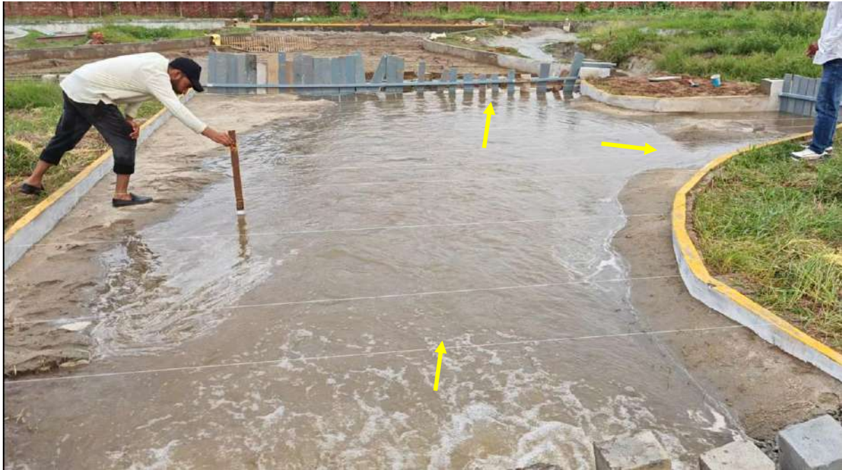
Fig. 8.7g Flow pattern for 41500 m 3 /s discharge under existing condition
